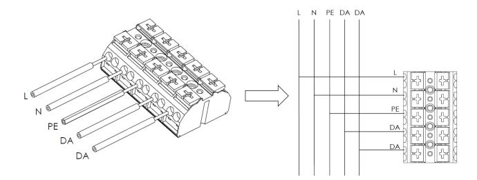
3 Phase connection (wiring 70):
